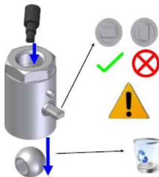
1. With a pick, carefully remove the second valve seat taking care not to scratch the internal surfaces of the valve. Discard the valve seat.
