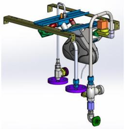
Compac Model Laser LPG Hydraulics Schematic Drawing – The Pattern
