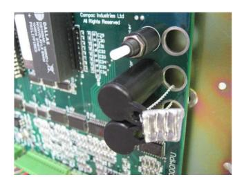
Typical Sealing Method for the Compac Model C4000 Processor PCB
