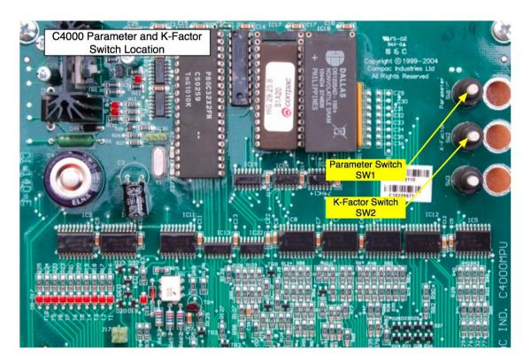
Figure 1: Parameter and K-Factor switches.
