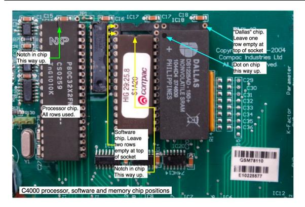
Figure 2: Processor, software and memory chip location.
