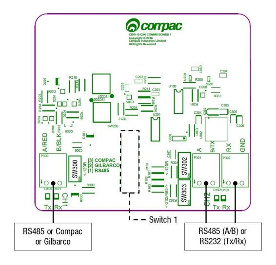
Switches 300, 302, and 303 are for RS485/RS232 Terminator application. Use the following table to configure these switches. Switch 300 is for channel 1, and switches 302 and 303 are for channel 2.
