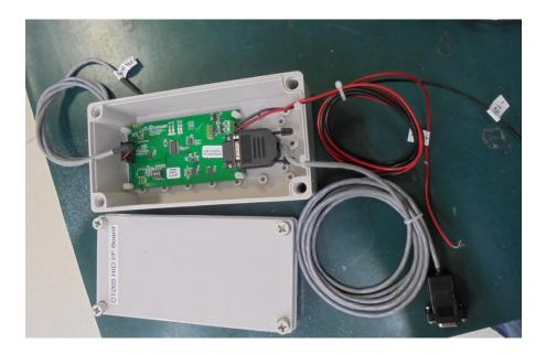
• Use UPS board CON7 Terminal to supply power to the Cl265-HID I/F Board.
