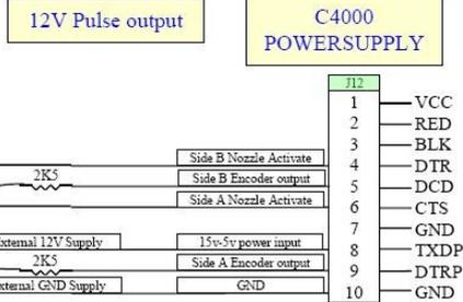
**⚠ NOTE** If a Triscan unit is not connected to the Pump or Dispenser, "Standalone operation" can be achieved by "shorting" Triscan Switch A (terminal "CTS"), & Triscan Switch B (terminal "DTR") to terminal "GND" & linking terminal "VCC" to terminal "TXDP". This must not be done if a Triscan unit is connected.
