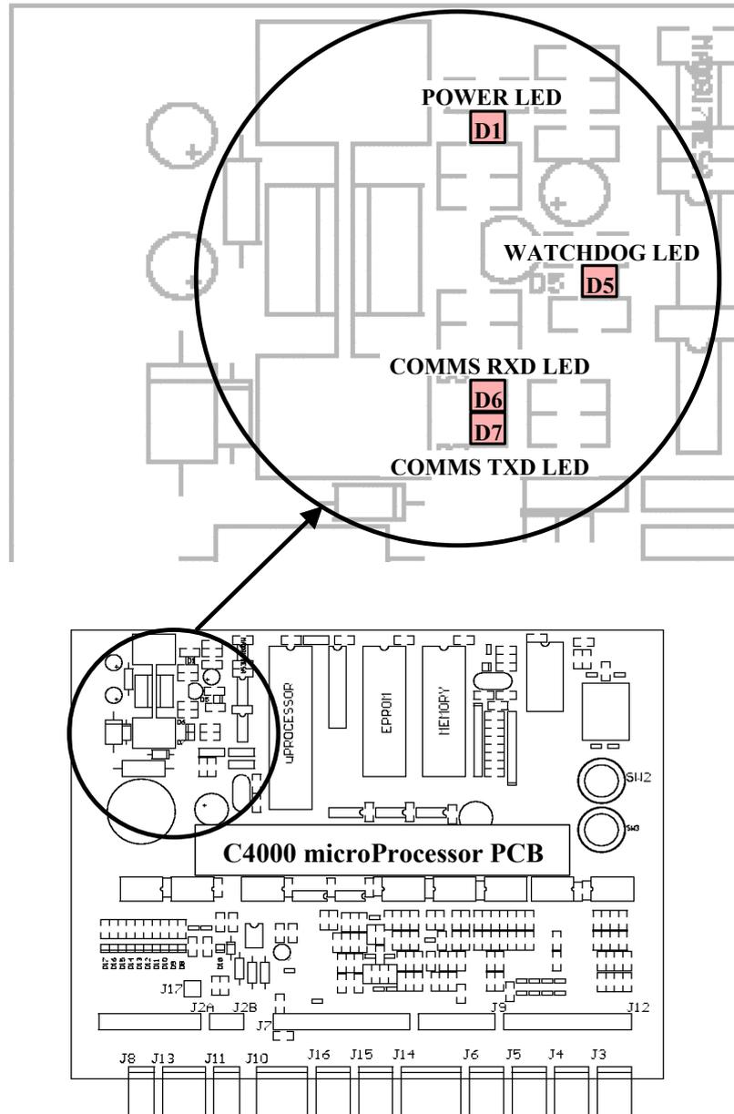
Figure 5. Location of Power, Watchdog, RXD & TXD LEDs
