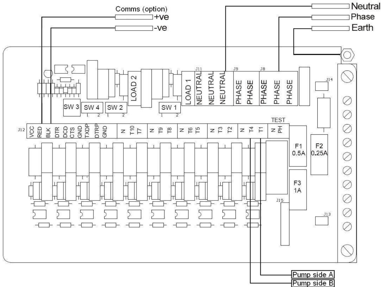
For single dispensers, wire pump contactor to T1 (230V Phase) only.
