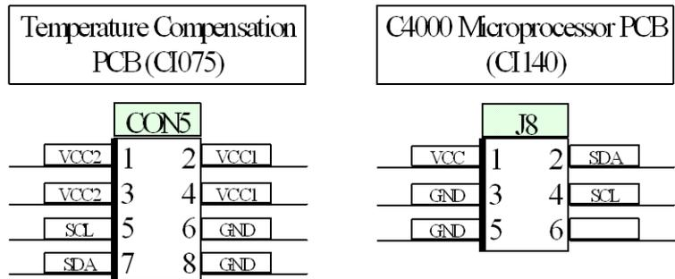
Figure 2: Temperature Compensation Connectors.
