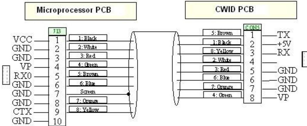
Figure 5: CWID (CON5) to microprocessor (J13) cable
