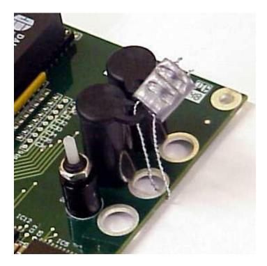
Typical Sealing of Meter Calibration (k-factor) Switch
