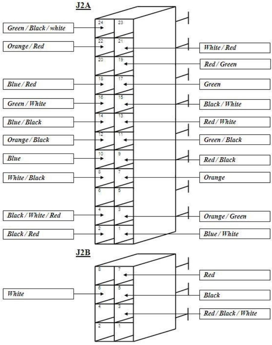
C4000 with RS485 MOD-BUS Wiring
