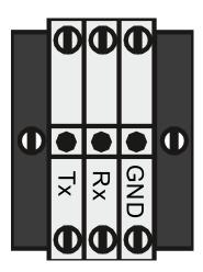
Cable length should be less than 3 metres. Cable length can be extended up to 10 metres if an opto-isolator is used.
