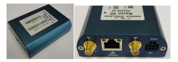
4) **Third Generation Call Direct** – This has a SMALL square power plug and two aerial connections (Only one is actively used)
